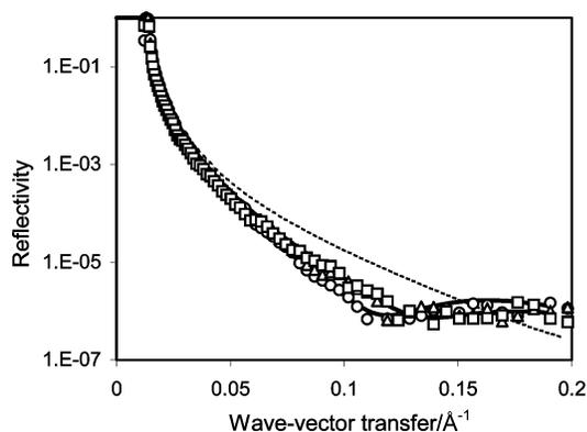
**Figure 6.** Extent of irreversibility of adsorbed peptide WWW15 as demonstrated by small changes in reflectivity profiles after rinsing under different pH. The peptide layer was adsorbed at pH 7 (○), followed by rinsing with pH 7 buffer (△), and subsequently pH 5 buffer (□) (0.01 wt %). The dashed line represents the reference D<sub>2</sub>O measurement.
