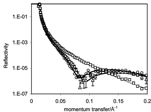
**Figure 5.** Reflectivity profiles measured at pH 5 (□), 7 (Δ), and 9 (○) for peptide WWW15. The dashed line represents the reflectivity measured from pure D<sub>2</sub>O buffer. The continuous lines are the three layer fits with their structural parameters listed in Table 1.
