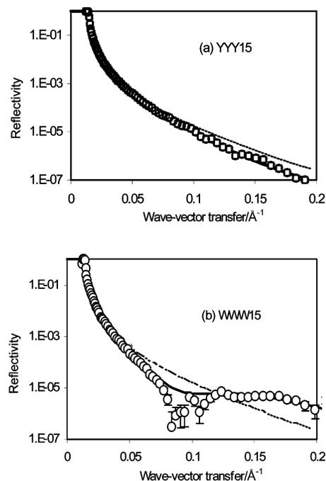
**Figure 2.** Reflectivity profile measured from the solid SiO<sub>2</sub>/D<sub>2</sub>O interface (dashed line) is compared with the ones from 0.1 wt % YY15 (a) and WWW15 (b) at pH 7. The continuous lines represent the best uniform fits with structural parameters listed in Table 1.
