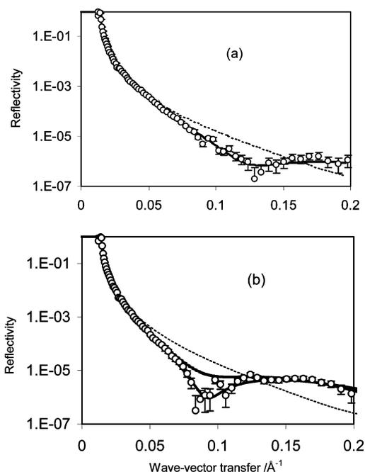
**Figure 4.** Neutron reflectivity measured from peptide WWW15 adsorbed at the SiO<sub>2</sub>/D<sub>2</sub>O interface with the peptide concentration at 0.01 (a) and 0.1 wt % (b). The reflectivity from the pH 7 D<sub>2</sub>O buffer is shown as dashed line for comparison. The continuous lines represent the best uniform layer fit in (a) and three layer model fit in (b). The long dashed line in (b) represents the best uniform layer fit.
